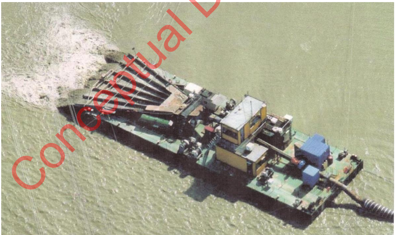
Figure 1-13: Sand Spreader Barge with Diffuser System
